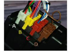
The positions and colors of the connectors are identical for the Siemens VDO and Stoneridge tachographs.
